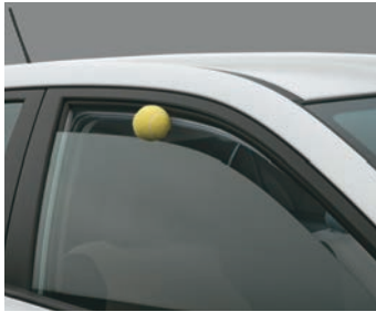
Auto Up/Down Power Window with Pinch Guard
