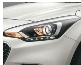
Projector Headlamps with LED DRL, Positioning and Cornering Lamps
