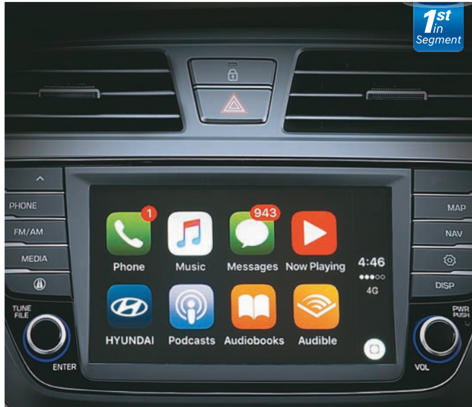
7.0 Audio Video Navigation System with Smartphone Connectivity (Apple CarPlay, Android Auto & Mirror Link)
