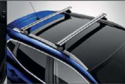
Cross bars for roof railing
