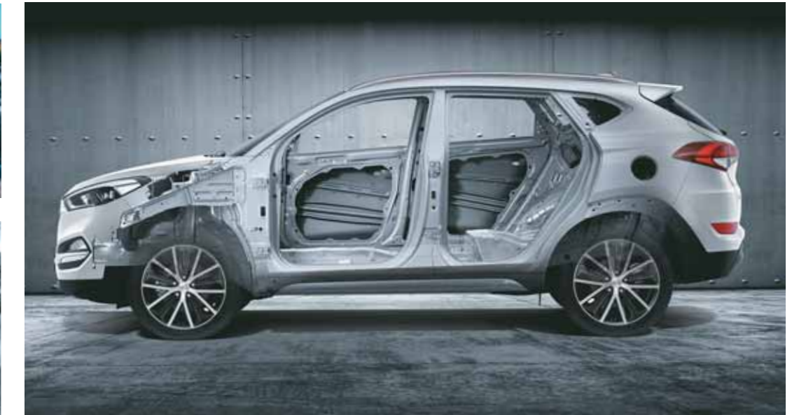
Strong structure with 51% Advanced High Strength Steel
