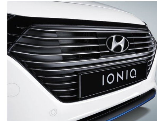
Efficient design: active air flaps in the grille open and close automatically in stages to enhance aerodynamic performance.
