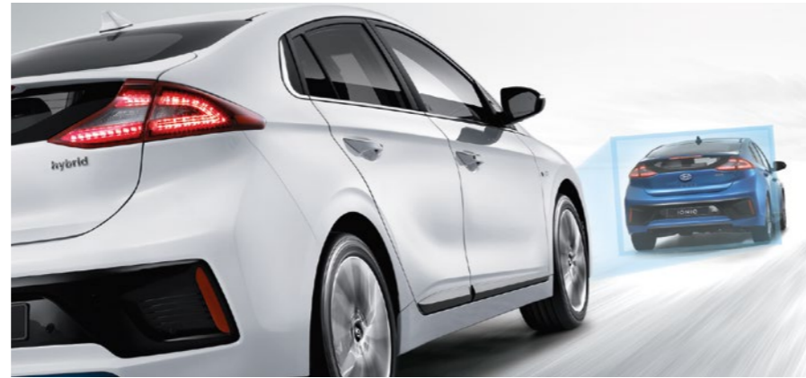
Autonomous Emergency Braking (AEB): when a potential collision with a vehicle or pedestrian is detected, AEB first gives a visual and an audible warning, then intervenes with partial or complete brake application.
